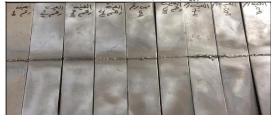
Fig. 3: MIG Welded specimens
