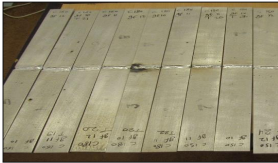
Fig. 5: TIG Welded specimens
