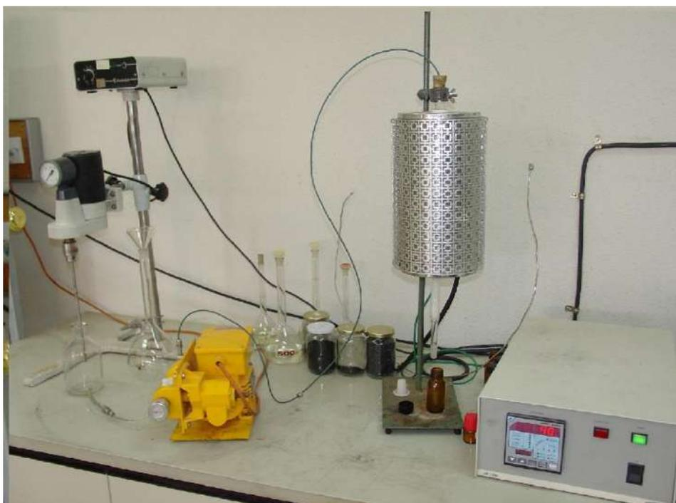
Figure 1: photograph of assembled apparatus used for adsorption.
