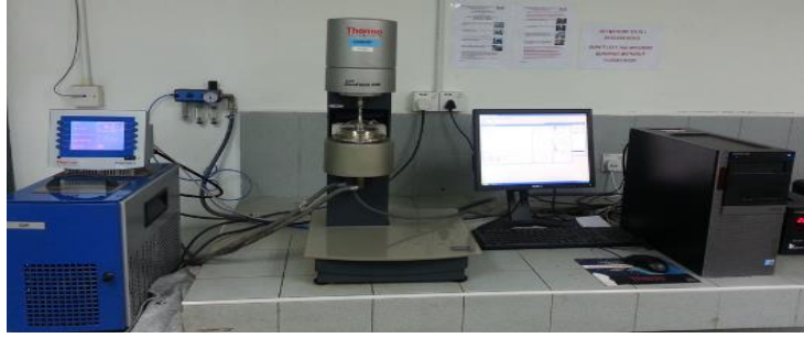
Fig. 4: DSR Equipment and Its Components
