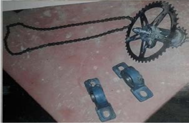
Figure 2: Bearing and sprocket wheel (transmission parts).
