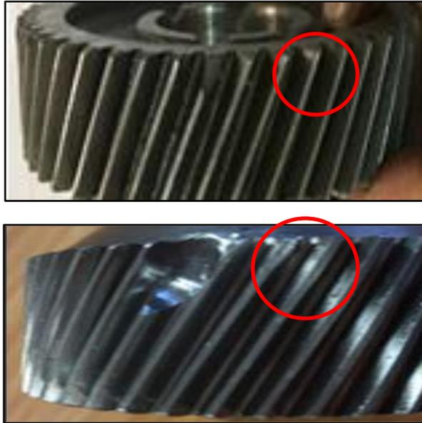
Fig.3: A photo of the helical gear under investigation with quarter tooth machined
