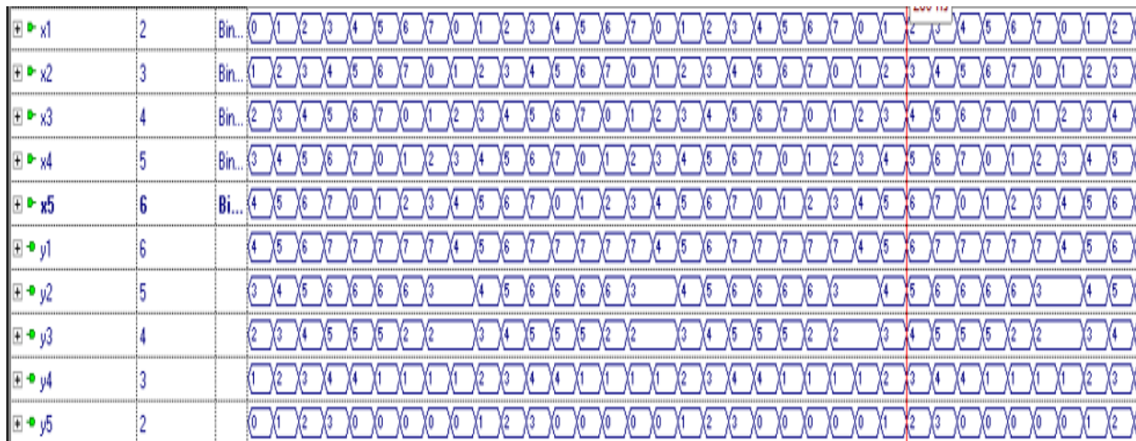
Figure 5: Waveform shows the Simulation of bubble sort implementation processor
