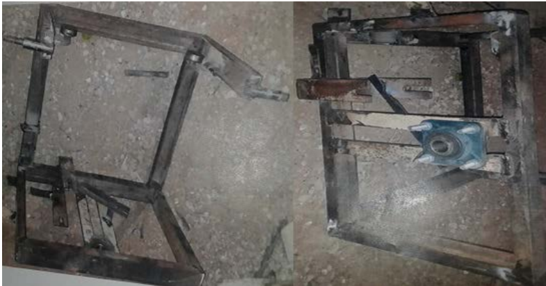
Figure 3: Fabrication of concrete mixer body.
