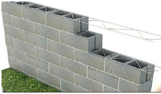
Fig. 5: shows the method of supporting the walls with an iron grid of diameter ( \varnothing 10mm)
