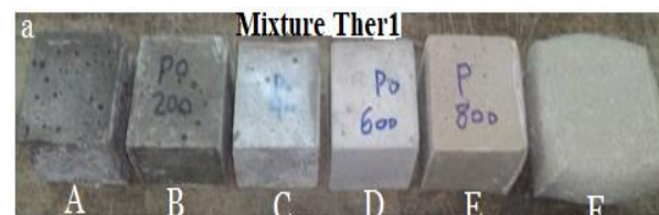
Figure 2 : Photographs of hardened single alkali activated mortars containing u-POFA Ther1, before and after being exposed to elevated temperature of (A) 28°C, (B) 200°C (C) 400°C (D) 600°C (E) 800°C (F)1000°C
