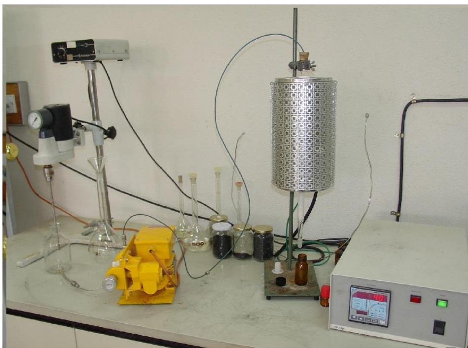
Figure 1: photograph of assembled apparatus used for adsorption.
