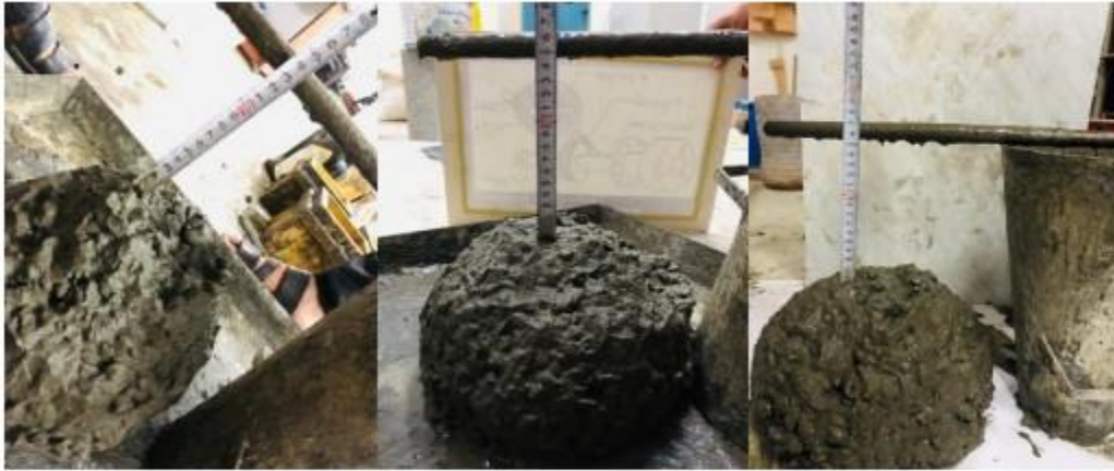
Plate 1: Slump test in progress
