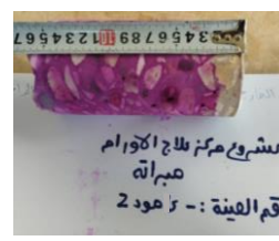
Fig. (19-2): Carbonation depth for Sample 2
