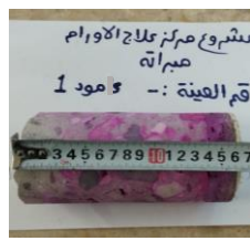
Fig. (19-1): Carbonation depth for Sample 1
