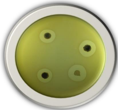
Figure: 3. Antibacterial activity of treated TiO 2 nano-composite prepared with 10% (m/m) CHxG against E. coli . It is clear that the test showed antibacterial activity.
