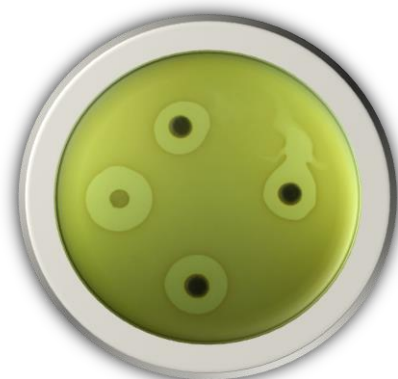
Figure: 6. Antibacterial activity of treated TiO 2 nano-composite prepared with 10% (m/m) CHxG tested against S. aureus . It is clear that the test showed antibacterial activity.
