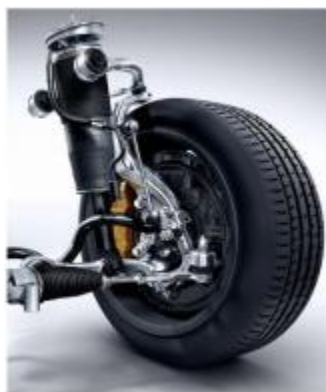
Figure 1 real quarter car suspension system
