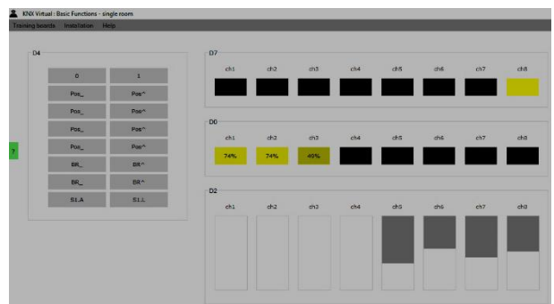
Fig. 38: meeting room simulation for each of the:1- switch actuator 2-dimming control 3-blind/shutter control.
