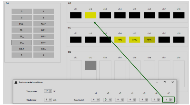
Fig. 21: bedroom 2 simulation for each of the: scenario control, binary input control (there is a fire).
