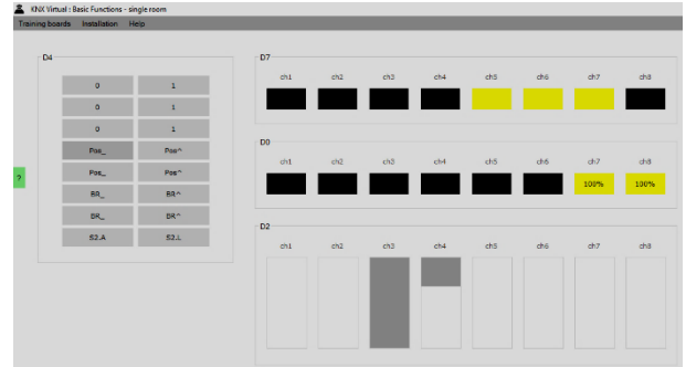
Fig. 29: living room simulation for each of the: 1-switch actuator 2-dimming control 3-blind/shutter control.
