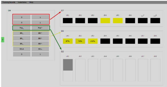
Fig. 17: bedroom 1 simulation for each of the: switch actuator, dimming control, blind/shutter control.
