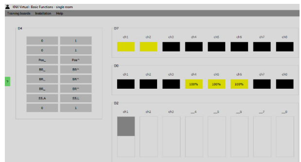
Fig. 23: bedroom 3 simulation for each of the: switch actuator, dimming control blind/shutter control.
