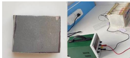
Fig. 1: The alloy specimen and setup preparation of anodizing cell
