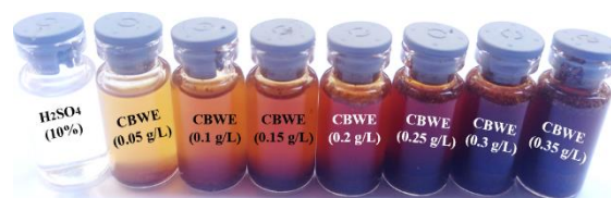
Fig. 5 Extraction Results of Inhibitor from Cigarette Butt Waste.
