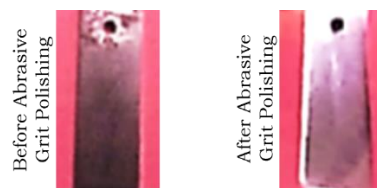
Fig. 1 The Weight Loss Test Specimens, Before and After Abrasive Grit Polishing.
