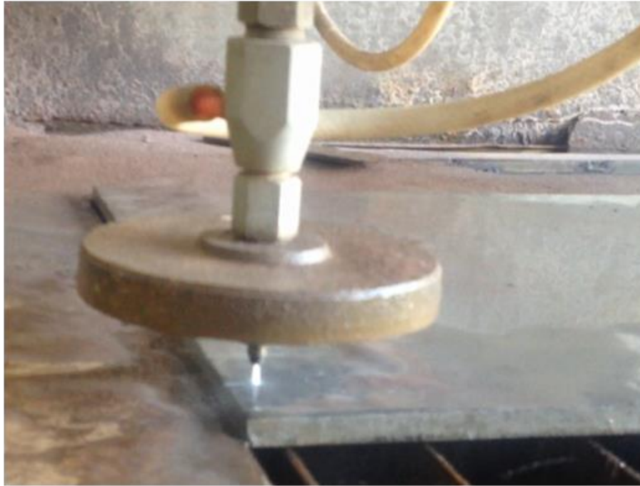
Figure 1: Photo of machine during water jet cutting process.
