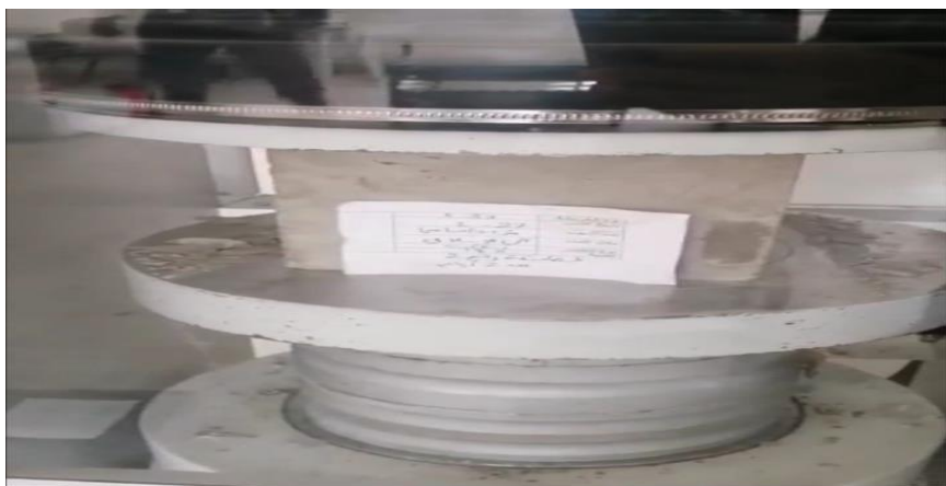
Figure 3 samples during testing in the compression machine
