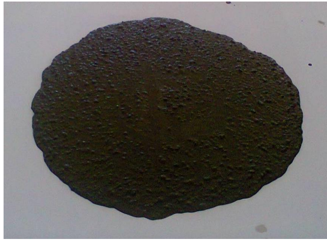
Figure (1) shape of the flow of concrete with a coarse aggregate percentage of 55%.
