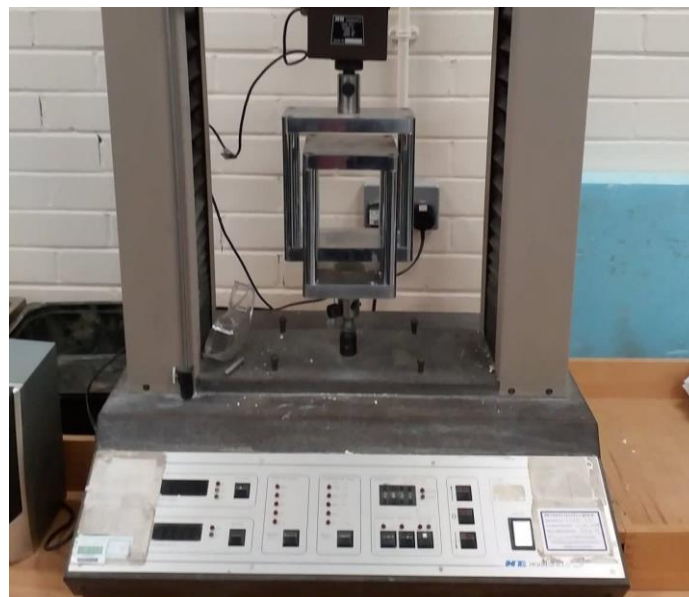
Fig.2: The 10kN capacity Hounsfield compression machine.
