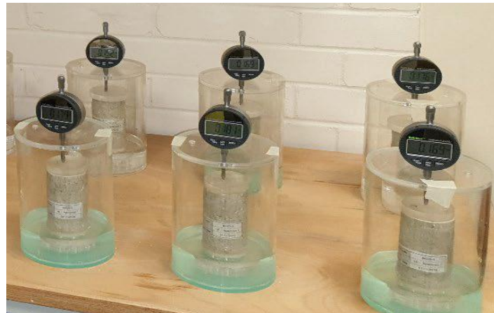
Fig.4: Linear expansion specimens under expansion measurement.
