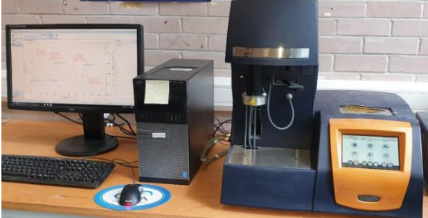
Fig.5: Thermogravimetric (TG) and derivative thermogravimetric (DTG) analyser used in this study (TGA55).
