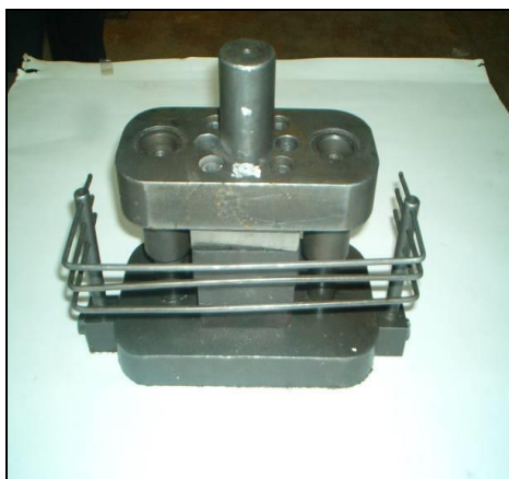
Fig. 7: The basic element of a blanking or piercing die.
