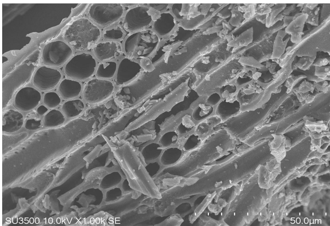
Figure 4.11. SEM micrograph of HCl-activated orange charcoal
