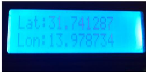
Fig. 17: Displays the coordinates on the LCD screen.
